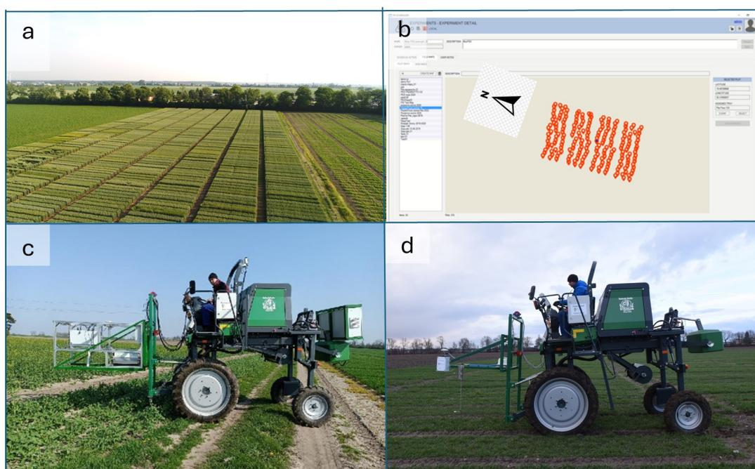
**Fig. 2** Field-Screen System (PSI) mounted on the Zurn 540 tool carrier, (a) view of the experimental fields where RGB phenotyping was carried out; (b) fragment of the field map with planned photo-taking locations. The arrow indicates the north direction; (c) entering the field through the sowing strip; (d) canopy density phenotyping.
