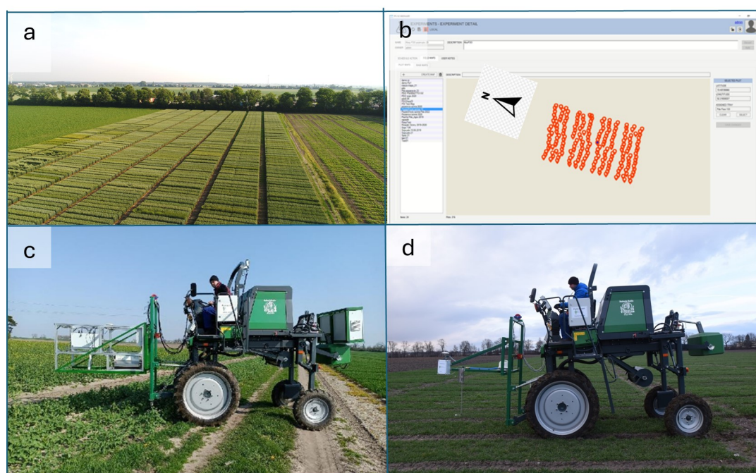
Fig. 2 Field-Screen System (PSI) mounted on the Zurn 540 tool carrier, (a) view of the experimental fields where RGB phenotyping was carried out; (b) fragment of the field map with planned photo-taking locations. The arrow indicates the north direction; (c) entering the field through the sowing strip; (d) canopy density phenotyping.
